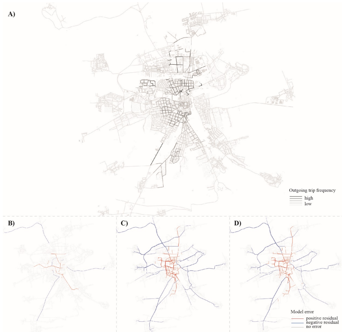
Figure 10a: Spatial distribution of the trip frequencies defined by the fully specified reference model M1. Figure 10b, c, d: Spatial distribution of model errors – residuals for b) M2 model, c) M3 model and d) M4 model. The amplitude of the error is expressed by the line thickness while the valence is defined by color (red = positive residuals, blue = negative residuals).
